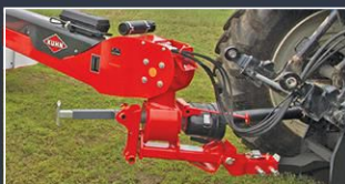
Standard drawbar or 2-point Gyrodine® swivel hitch for tight turns
